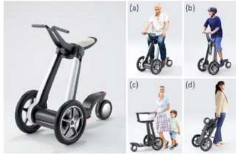
Fig. 1 Developed Personal Mobility: ILY-A (a) Normal Vehicle Mode, (b) Standing/Kicking-Ride Mode, (c) Cart Mode and (d) Carry Mode
