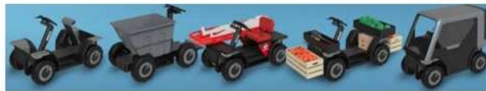
Fig. 1 Developed Personal Mobility: ILY-A (a) Normal Vehicle Mode, (b) Standing/Kicking-Ride Mode, (c) Cart Mode and (d) Carry Mode
